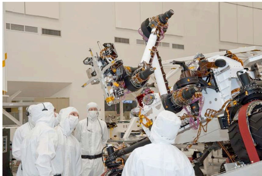
FIGURE 1.7 Mars Science Laboratory Curiosity rover undergoing a test of its sample arm while on a tilt table at the Jet Propulsion Laboratory in September 2010. SOURCE: NASA/JPL-Caltech.
